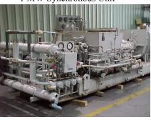
A 1 MW condensing unit is fueled by scrap wood helping a crate manufacturer reduce it's total energy costs.
